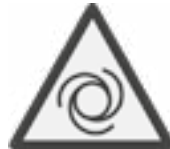
Machinery starts automatically
