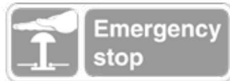
Emergency stop for machinery
