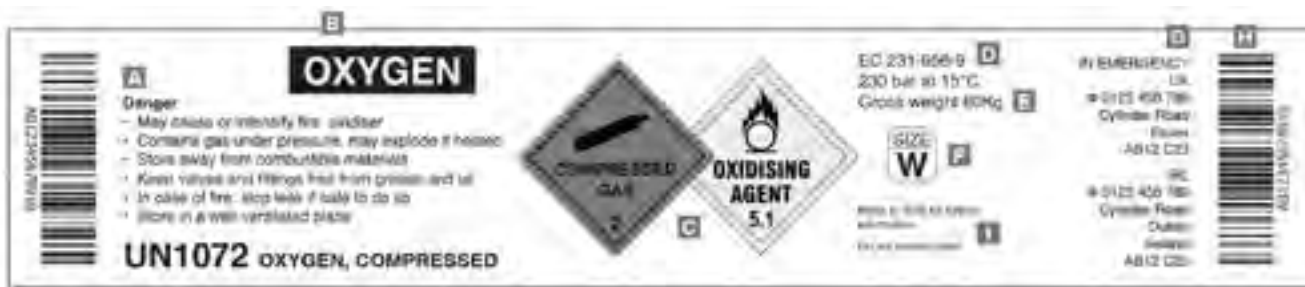
A Hazards and precautions, B Name of product, C Hazard (flammable), D Filled pressure, E Gross weight, F Cylinder size, G Contact information, H Unique cylinder serial number, I Additional company information
