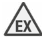
Danger Explosive atmosphere
